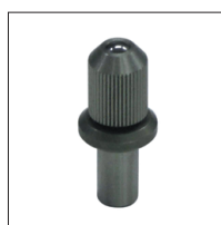
Tungsten carbide ball indenter of φ 5mm for Brinell
