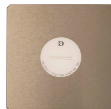
Stage micrometer (for verifying Brinell measuring microscope)
